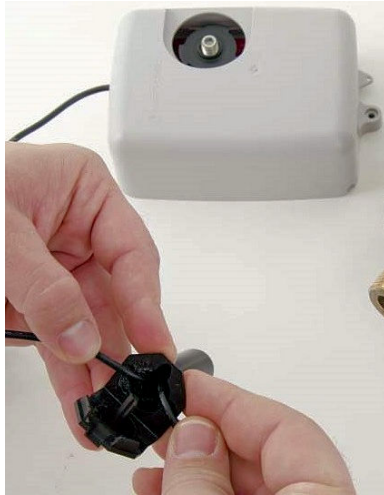
Figure 11 – Gray Wires in Slot
